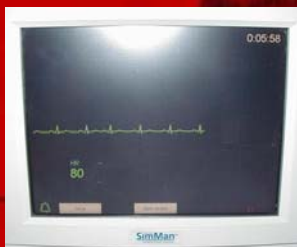
Picture 1: Laerdal SimMan patient monitor with ECG signal and pulse rate repositioned and its VGA output connected to a data projector.
